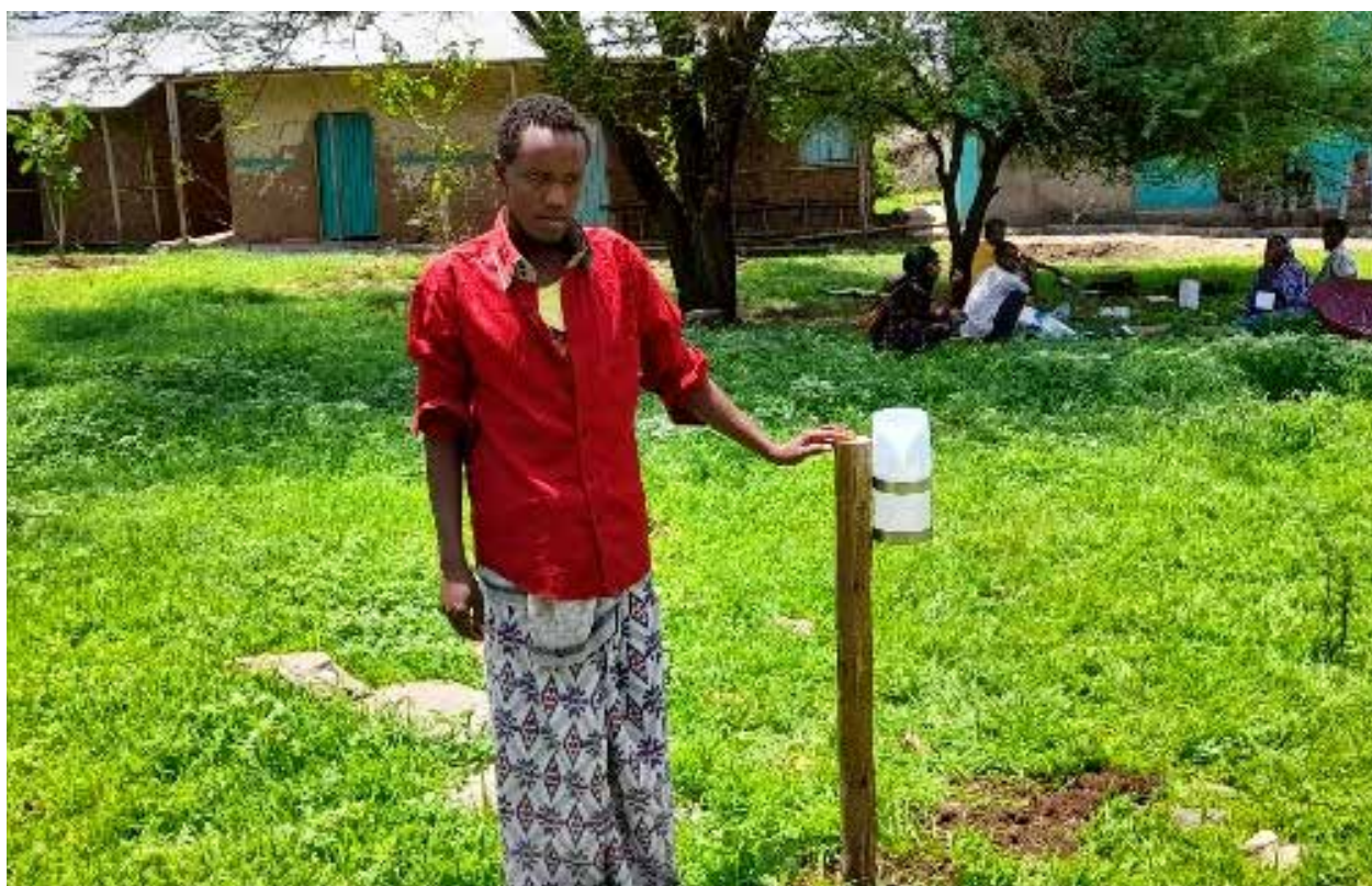
A man showing a plastic rain gauge installed by the Gari Iffebas FS members
